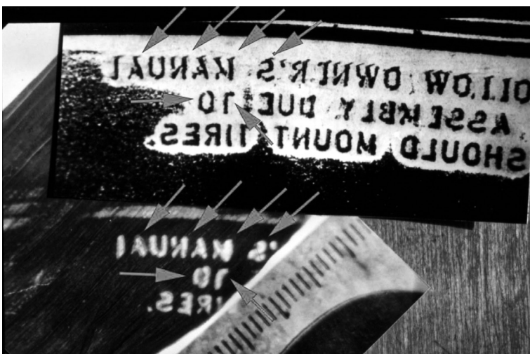
Photo 10. Individual characteristics of the rubber letters were reflected on the paper sheet and the corn leaf
