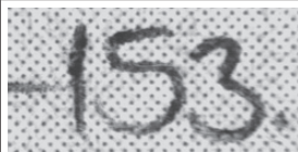
Fig. 4. Fragment of questioned entry “1” in the examined document in space “Należn.” (“Amount due”) in long-wave (365 nm) ultraviolet light at maximum magnification of VSC 2000/HR.
