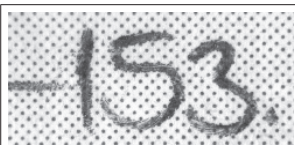
Fig. 3. Fragment of questioned entry “1” in the examined document in space “Należn.” (“Amount due”) in white light enriched with infrared radiation at maximum magnification of VSC 2000/HR.
