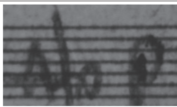
Fig. 12. Fragment of questioned entry "sto" in the examined document in long-wave (365 nm) ultraviolet light at maximum magnification of VSC 2000/HR.
