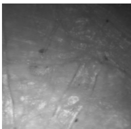
Figure 28. “Black dots” in the paper structure of the examined document
